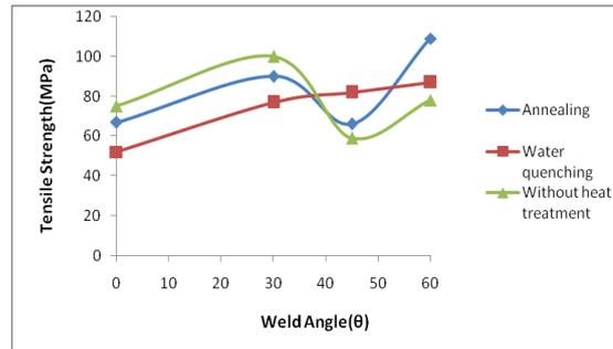
Fig. 2 Tensile specimens under annealing (A), water quenching (WQ) and without heat treatment (WH)
