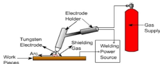
FIG. 1 TIG WELDING SYSTEM SETUP
